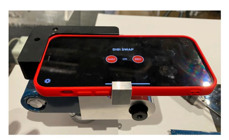
If the knob screw of 6 is loosely tightened, the smartphone will come off.
